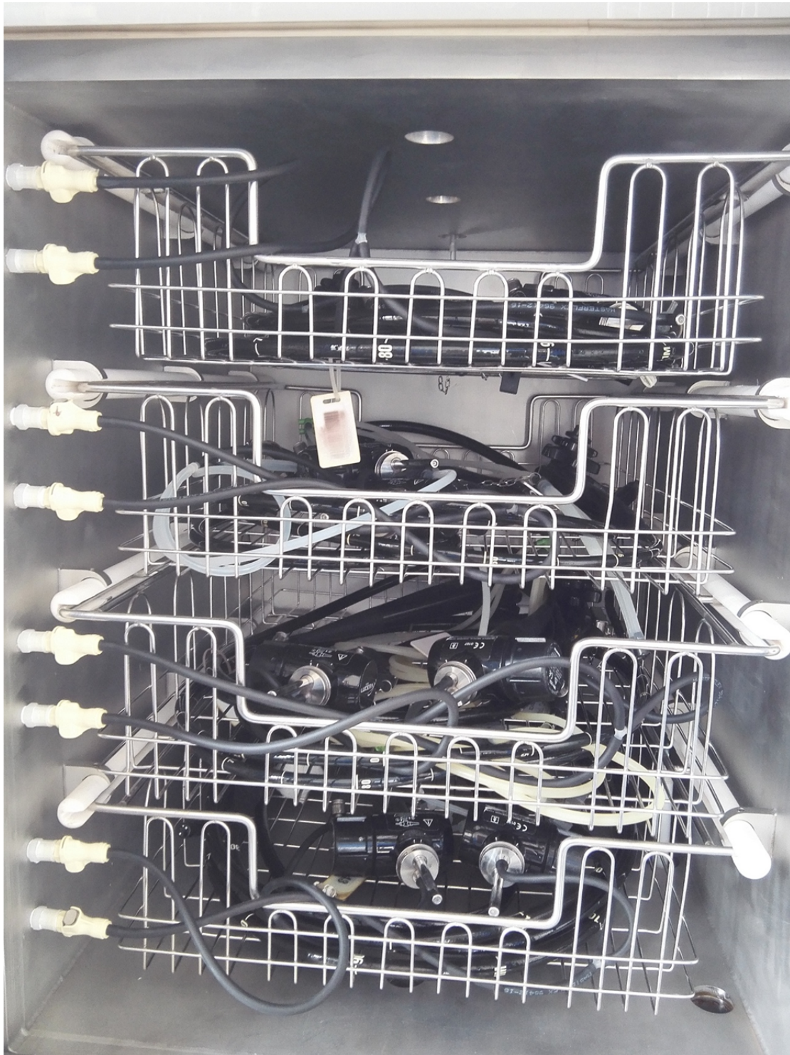
Figure S2 Six gastroscopes (GIF-Q260, Olympus, Japan) and two colonoscopes (CF-Q260AI, Olympus, Japan) to be disinfected in the experimental prototype
