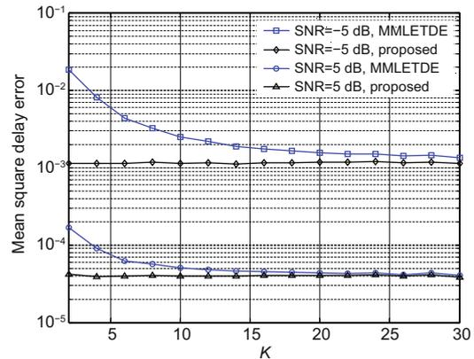
Fig. 7 Steady-state performance with  $2 \leq K \leq 30$  for sinusoidal signals ( $\mu = 1.0 \times 10^{-4}$ )
