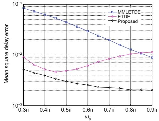
Fig. 6 Steady-state performance with different center frequencies (SNR = -5 dB,  $K = 2$ )
