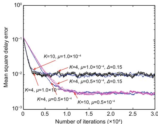
Fig. 2 Learning curves with different parameter settings for sinusoidal signals (SNR=-10 dB)
