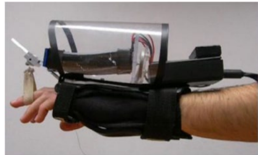
Fig. 3 A DE actuator for hand rehabilitation (Reprinted from Carpi et al. (2008), Copyright 2008, with permission from SPIE)
