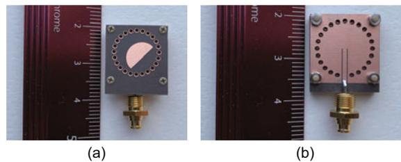
Fig. 8 Fabrication of the proposed antenna: (a) top view; (b) bottom view
