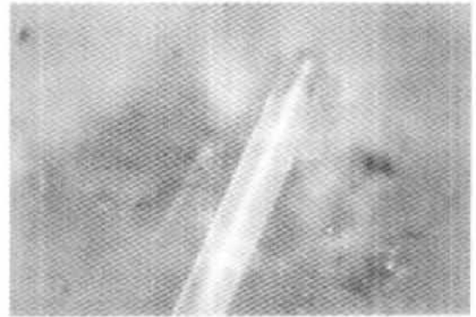
Fig. 7 Typical glass fiber (batch # 3) in the optical microscopic image (500 ×)
