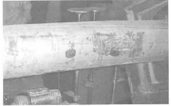
Fig.7 The failure modes in torsion and bending
