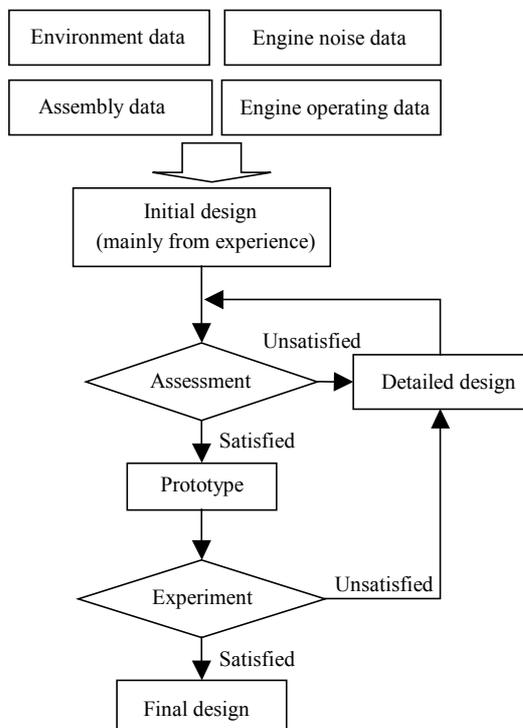
Fig.1 Typical process of design and development of an intake system
