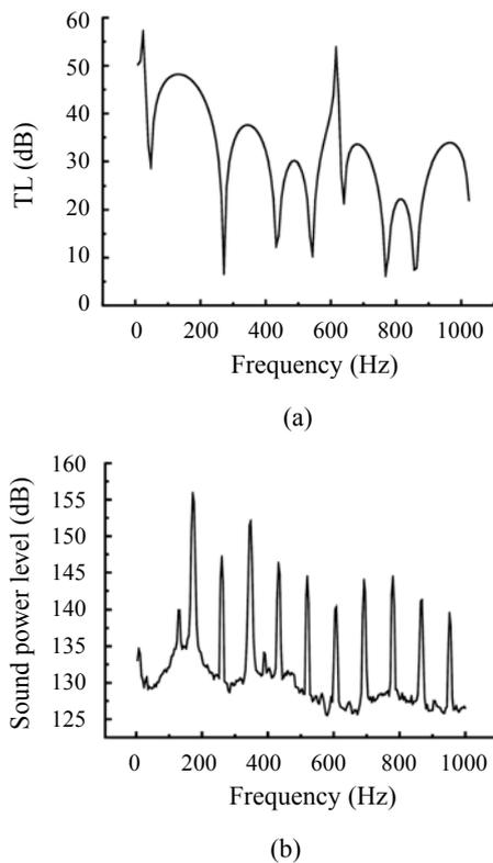
Fig.3 Transmission loss of original air cleaner (a) and sound power level at engine intake port (b)
