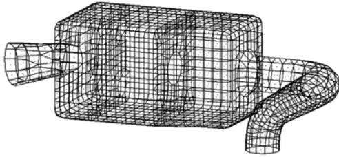
Fig.6 BEM mesh of the silencing air cleaner
