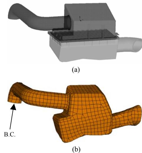
Fig.2 CAD model (a) and BEM mesh (b) of original air cleaner
