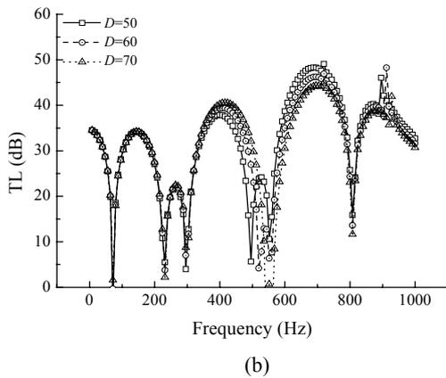
Fig.7 TL respectively when  $L_1=145, 155, 165, 175$  mm (a) and TL respectively when  $D=50, 60, 70$  mm (b)
