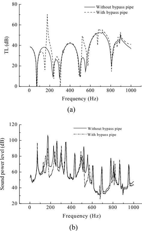
**Fig.10** TL (a) and sound power level (b) of air cleaners with and without bypass pipe at the main pipe
