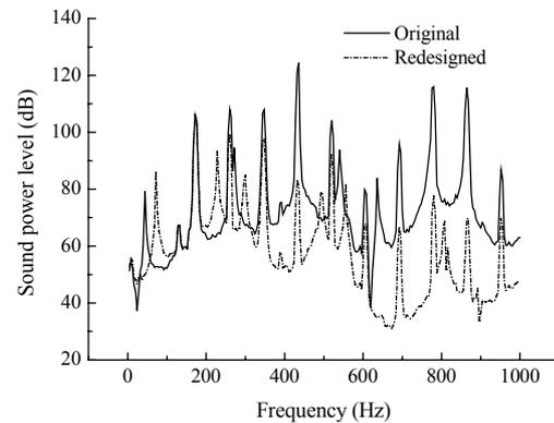
Fig.8 Sound power level of the original and the redesigned air cleaner's intake noise
