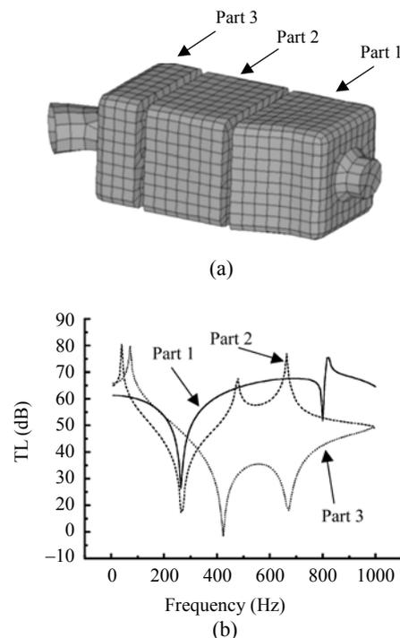
Fig.5 Three parts of the air cleaner (a) and TL of the three parts (b)
