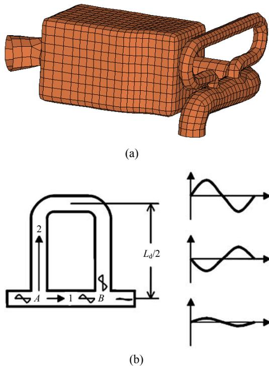
**Fig.9** Air cleaner with bypass pipe (a) and theoretical effect of bypass pipe (b)
