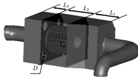
Fig.4 Layout of the initial design of the silencing air cleaner
