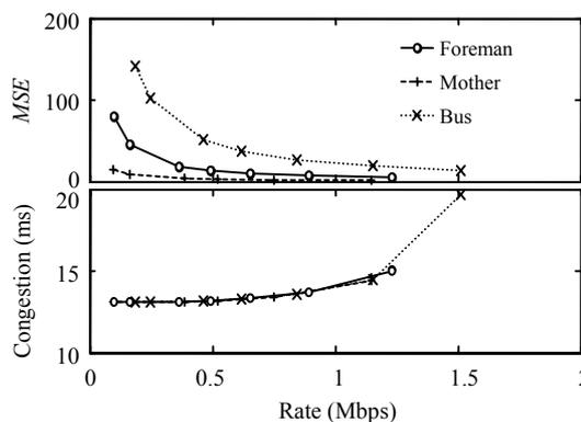
**Fig.3 Trade-off between network congestion in terms of average link delay and video distortion in MSE resulting from the joint routing and rate allocation scheme, when streaming a single video sequence over the network**
