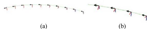
Fig.1 Step 1: (a) Discrete points P_0, P_1, P_2, \dots, P_{m-1} on the trajectory and corresponding reference frames on the points; (b) Magnified end of the trajectory
