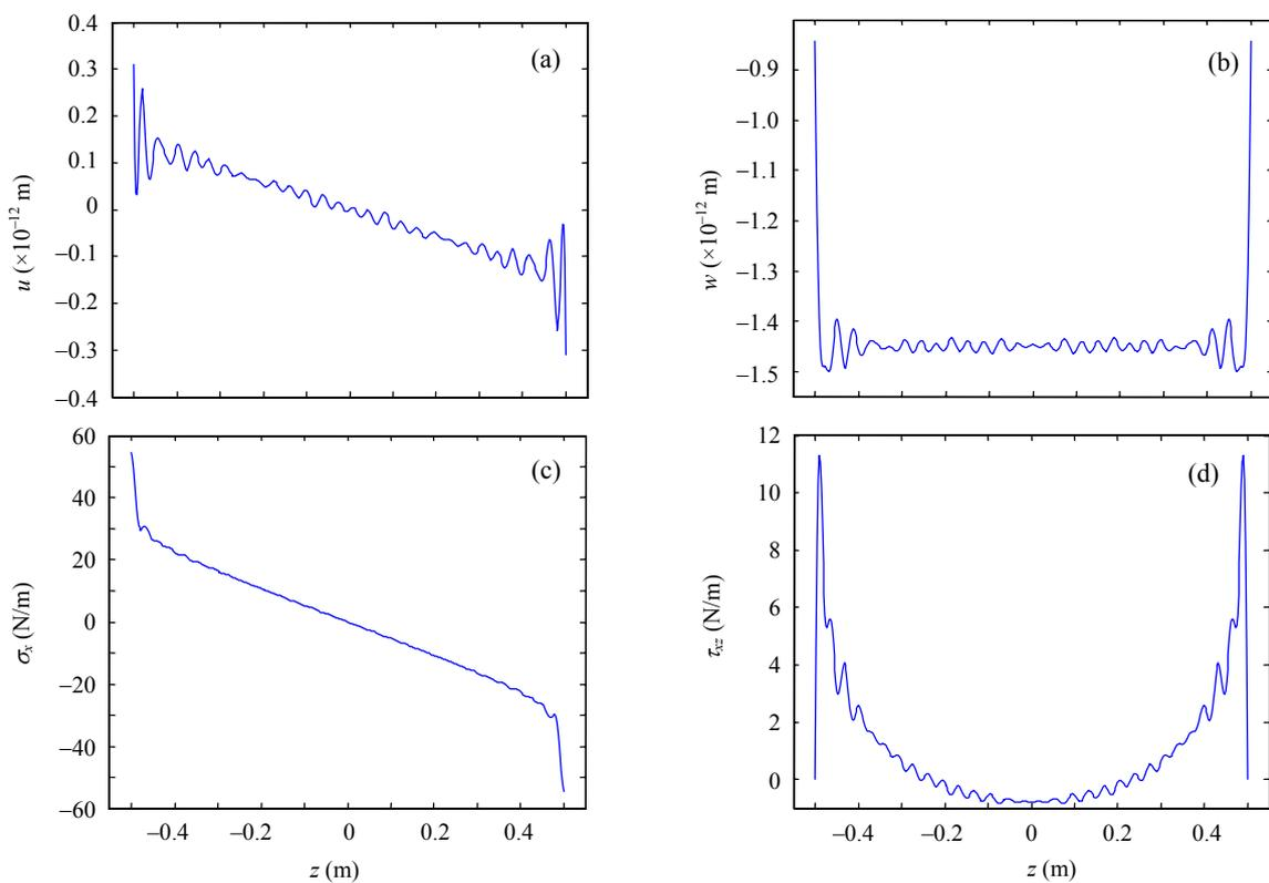
Fig.3 Stresses and displacements at the clamped end by discarding the  $\beta$ -set in Eq.(15). (a)  $u$ ; (b)  $w$ ; (c)  $\sigma_x$ ; (d)  $\tau_{xz}$
