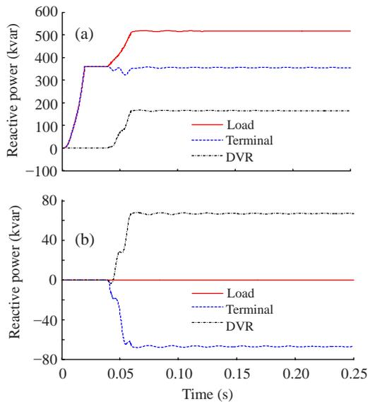
**Fig.10** Reactive power variation with a  $45^\circ$  injected voltage phase angle. (a) Case 1; (b) Case 2
