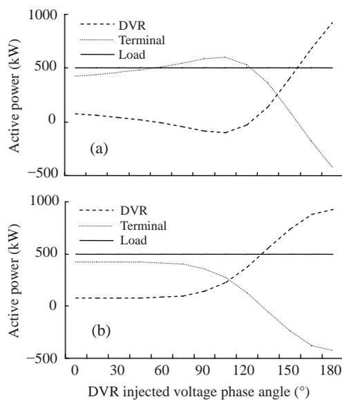
**Fig.8 Active power variation with injected voltage phase angles.** (a) Case 1, inductive load; (b) Case 2, resistive load
