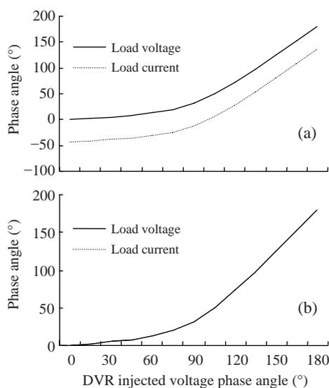
**Fig.7 Phase angle variation of load voltage and current with injected voltage phase angles.** (a) Case 1, inductive load; (b) Case 2, resistive load
