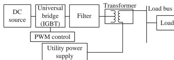
**Fig.3 Block diagram showing DC source as DG injecting voltage in series with utility supply**
