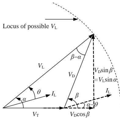
Fig.2 Phasor diagram of a system with leading voltage injection
