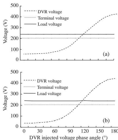
**Fig.4 Voltage variation with injected voltage phase angles**
