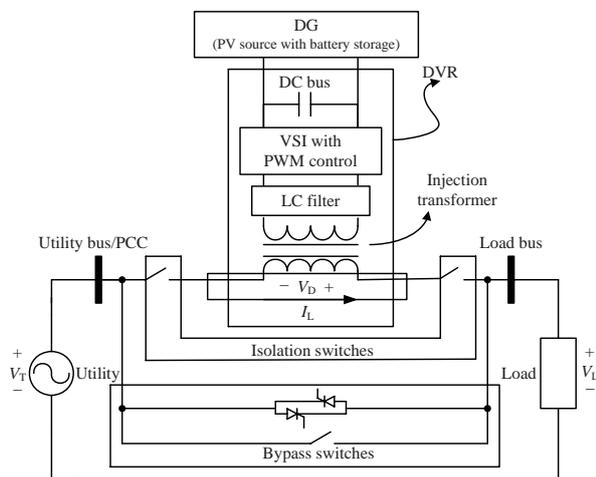
**Fig.1 Conceptual diagram of one phase of a dynamic voltage restorer (DVR) with its protection components**
