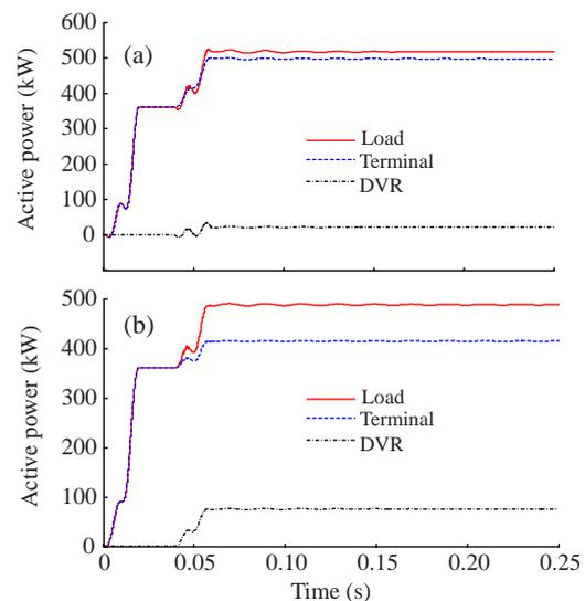
**Fig.9 Active power variation with a 45° injected voltage phase angle.** (a) Case 1; (b) Case 2
