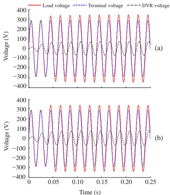
**Fig.6 Dynamic voltages with a 45° injected voltage phase angle.** (a) Case 1; (b) Case 2. 85% sag is initiated at 0 s and persists for 0.25 s (12.5 cycles)
