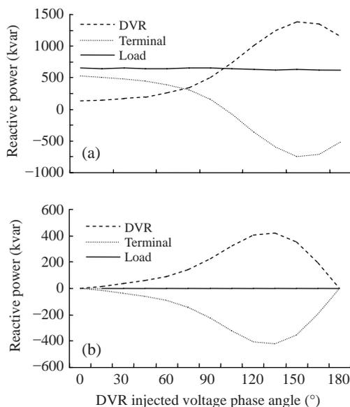
**Fig.11** Reactive power variation with injected voltage phase angles. (a) Case 1, inductive load; (b) Case 2, resistive load
