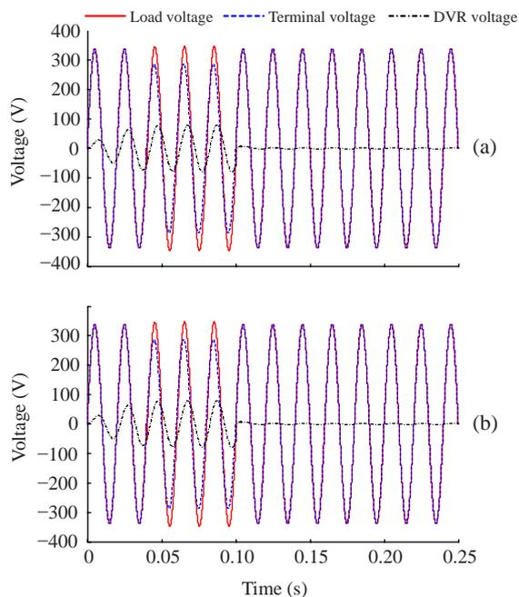
**Fig.5 Dynamic voltages with a 45° injected voltage phase angle.** (a) Case 1; (b) Case 2. 85% sag is initiated at 0.04 s in the utility voltage which is kept until 0.1 s, with a duration of 0.06 s
