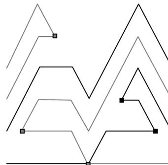
Fig.2 Topology of the arrangement  $f=0$  (gray) and  $g=0$  (black). Solid boxes represent the event points of the arrangement
