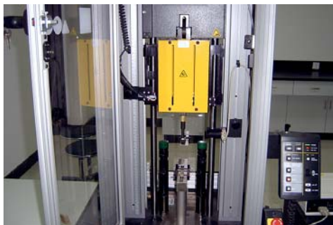
Fig. 11 The impact experiment instrument
