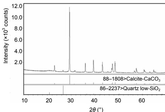
**Fig. 1 XRD-spectrum of the raw tannery sludge sample**
