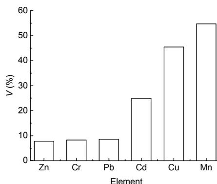
**Fig. 6 Vaporization fraction of heavy metals at 500 °C**
