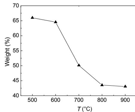
**Fig. 4** Weight loss during tannery sludge combustion in tube furnace
