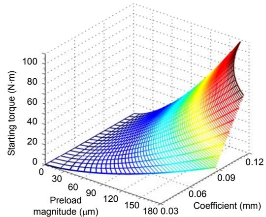
**Fig. 8** Theoretical relationship among the starting torque, the preload magnitude and the coefficient of rolling frictional resistance
