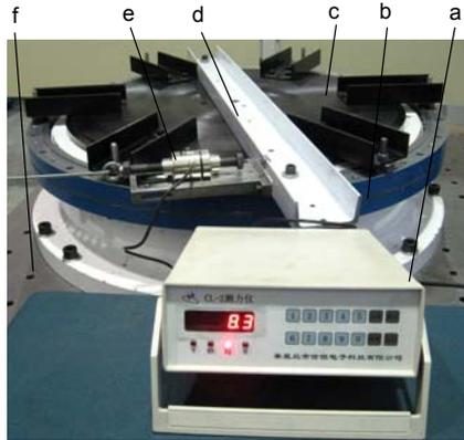
a: dynamometer; b: wire race ball bearing; c: rotating disc; d: steel channel beam; e: force transducer; f: experimental bench
