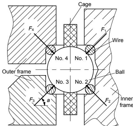
**Fig. 3 Schematic drawing of the contact status**
