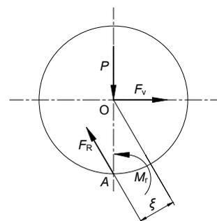
**Fig. A3 Sketch of the physical meaning for the coefficient of rolling frictional resistance**
