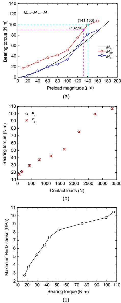
**Fig. 9** Theoretical and experimental results regarding the relationship between bearing torques and the preload magnitude, contact loads, and the maximum Hertz stresses (a) Theoretical and experimental bearing torques vs. the preload magnitude; (b) Experimental bearing torques vs. contact loads; (c) Experimental bearing torques vs. the maximum Hertz stresses of the contact point.  $M_{sc}$ : calculated bearing torque;  $M_{bm}$ : measured bearing torque;  $M_{sm}$ : measured starting torque
