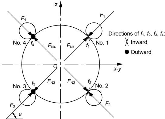
**Fig. 4 Equivalent drawing of the space force couple for the contact between one ball and four wire races**
