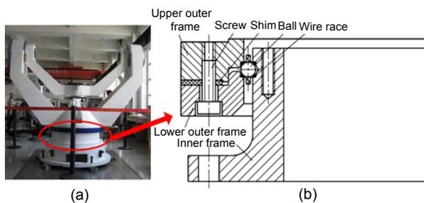
**Fig. 1** Wire race ball bearing used in aircraft simulating rotary table
