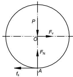
**Fig. A1 Sketch of the force diagram for a ball**
