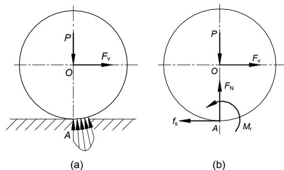
**Fig. 2** Sketch of the rolling frictional resistance
