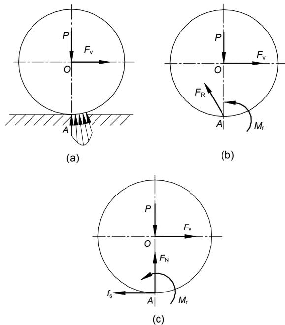
**Fig. A2 Sketch of the rolling frictional resistance** (a) Contact deformation zone; (b) Simplified force and the moment of rolling resistance couple; (c) Decomposition of force
