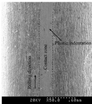
Fig. 10 SEM picture of the contact indentation on the contact surface of a wire race
