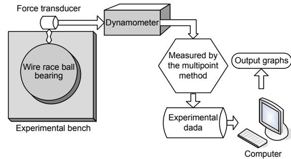
**Fig. 5 Diagrammatic sketch of the measurement system for the starting torque**
