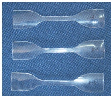
Fig. 1 Poly(ethylene terephthalate) specimens for tensile testing
