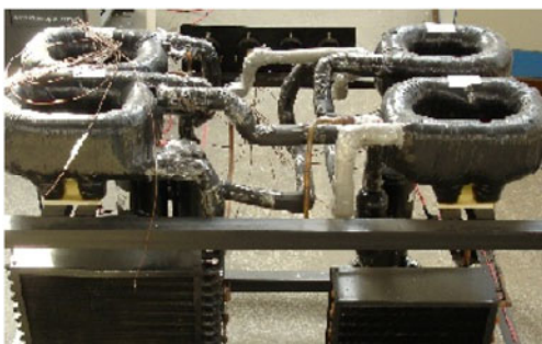
Fig. 2 Experimental apparatus of the dual-mode cascade refrigeration cycle
