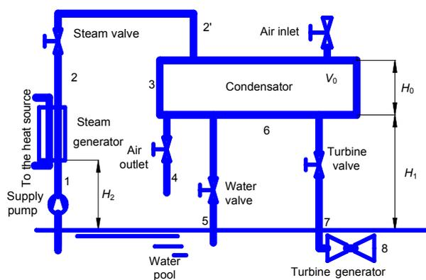
**Fig. 1** Schematic of the new power generation system  $H_0$  is the height of the condenser,  $H_1$  is the altitude of the condenser to the water pool, and  $H_2$  is the altitude of the steam generator to the water pool
