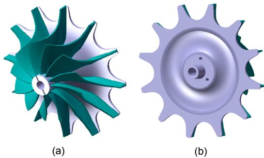
**Fig. 1** 3D geometric modeling of the final design wheel
