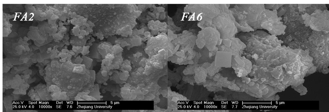
**Fig. 1 SEM images of fly ash samples (FA2 and FA6)**
