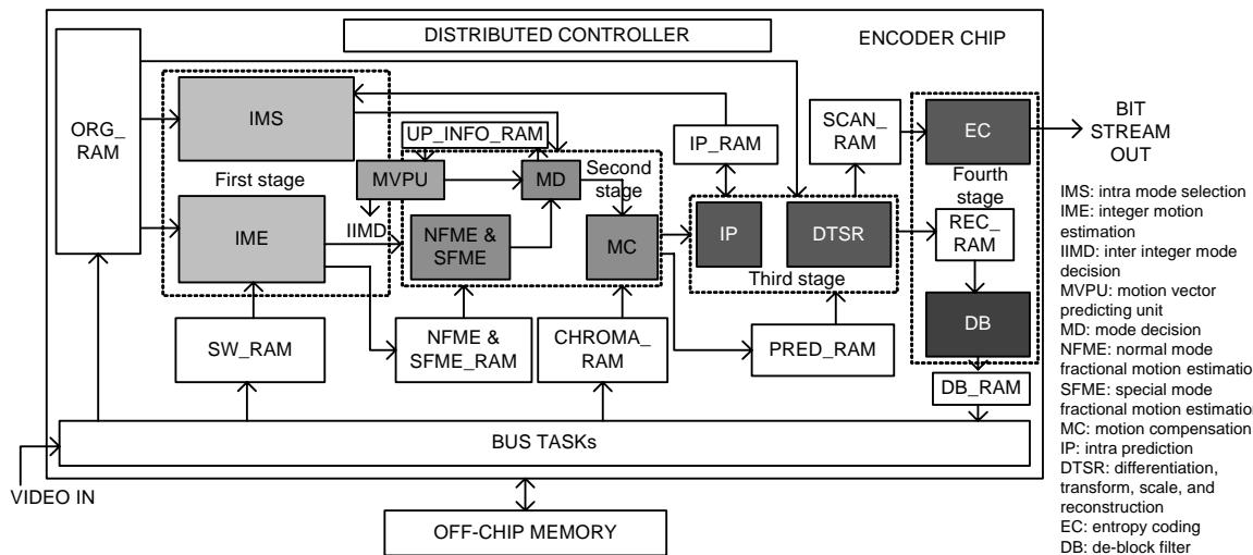
**Fig. 1** The proposed hardware oriented H.264/AVC HDTV encoder system
