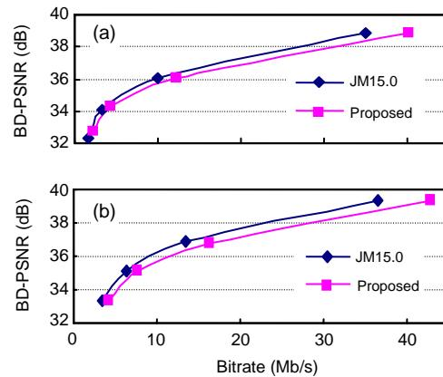
**Fig. 10 Rate-distortion curves of the proposed encoder and the reference software JM15.0**
