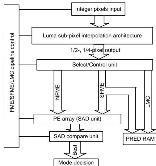
**Fig. 6** The proposed architecture of normal mode fractional motion estimation (NFME), special mode fractional motion estimation (SFME), and luma motion compensation (LMC)
