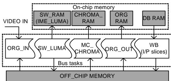
**Fig. 9 Bus tasks after data reuse**
