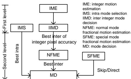
Fig. 4 The proposed two-level mode decision mechanism
