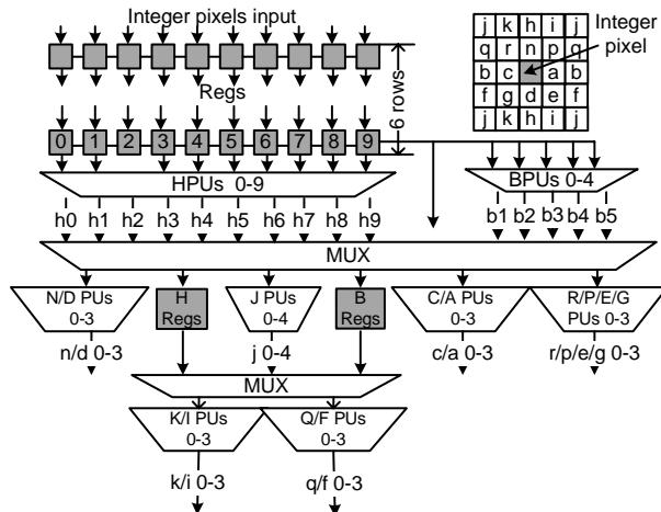
**Fig. 7** The proposed luma sub-pixel interpolation architecture and the diagram of all sub-pixels in different positions
