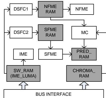
**Fig. 8** Data reuse of on-chip memory
