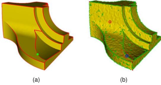
**Fig. 2 Neighbor supporting.** (a) represents a vertex lying on a feature line. In (b) a noisy vertex located in a circle has no support from neighbors. A real feature vertex located in a circle has a strong support from the line neighbors marked by a dotted ellipse
