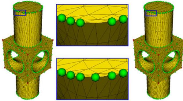
**Fig. 3** Feature detection results with different weights. Left and right pictures are the detection results of the mechanical part using the weights of Eqs. (4) and (6), respectively. The close-up of the detection results are shown in the middle pictures
