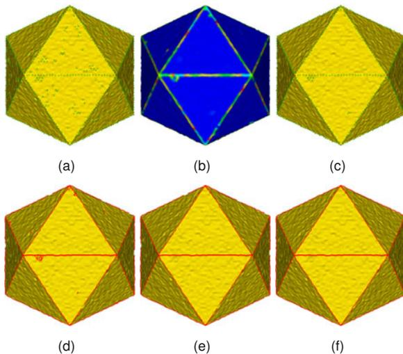
**Fig. 5 Branch pruning.** (a) Initial detected feature vertices; (b) Color map of the salient measure; (c) Feature vertices after filtering; (d) Initial feature lines; (e) Feature lines after branch pruning; (f) Final feature lines
