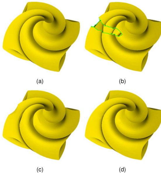
**Fig. 12** Feature-preserving hole-filling. (a) Octa-flower model; (b) A hole with sharp features missing; (c) Result of Chen and Cheng (2008); (d) Result of Wang et al. (2012) using the detected features
