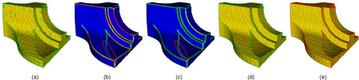
Fig. 1 Method overview. (a) is the initial feature vertex detection on a noisy Fandisk model. Sharp edge and corner type vertices are shown in different colors. (b) and (c) are the color maps of salient measure before and after weak feature enhancing, respectively. The weak features at the top of the fan are marked by an ellipse. (d) and (e) are the final detected feature vertices and feature lines, respectively
