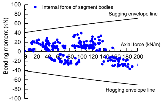
Fig. A1 Axial force and bending moments in the segments in the IT
