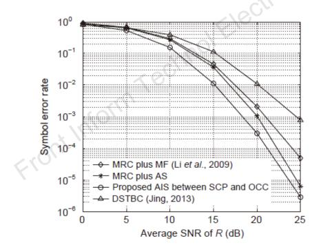
Fig. 5 Curves of the symbol error rate versus the average  $SNR_R$  with 16-QAM ( $SNR_D = SNR_R$ )
