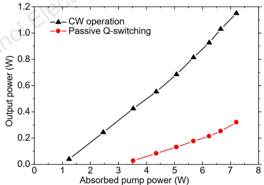
**Fig. 3** Output power and absorbed LD pump power
