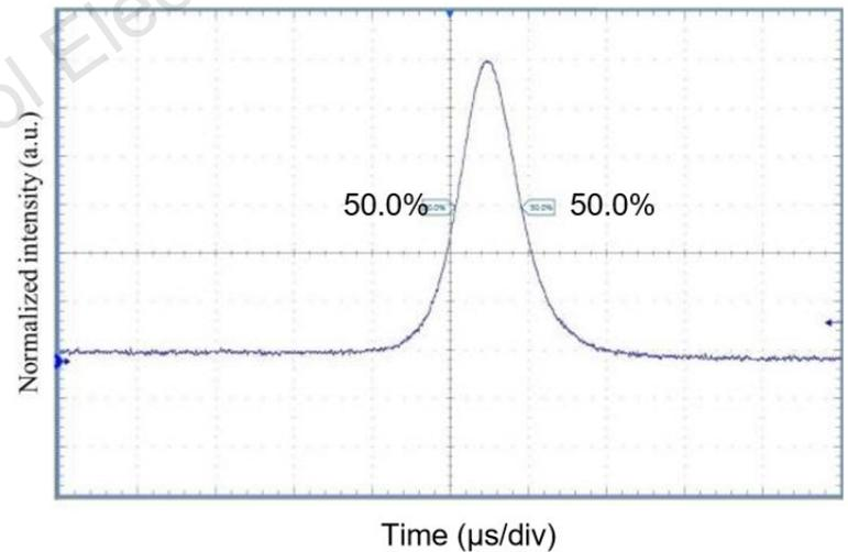
**Fig. 6** Shape of the 843 ns pulse
