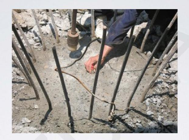
Low strain reflected wave signal detection method
