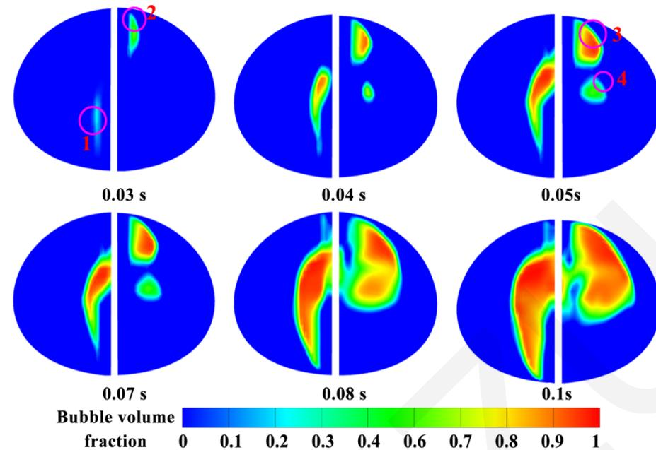
**Fig. 2** Bubble volume fraction evolution cloud over time on the flow surface.
