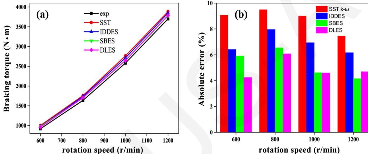
**Fig. 1** Comparison studies between the simulation and experimental data for different models.
