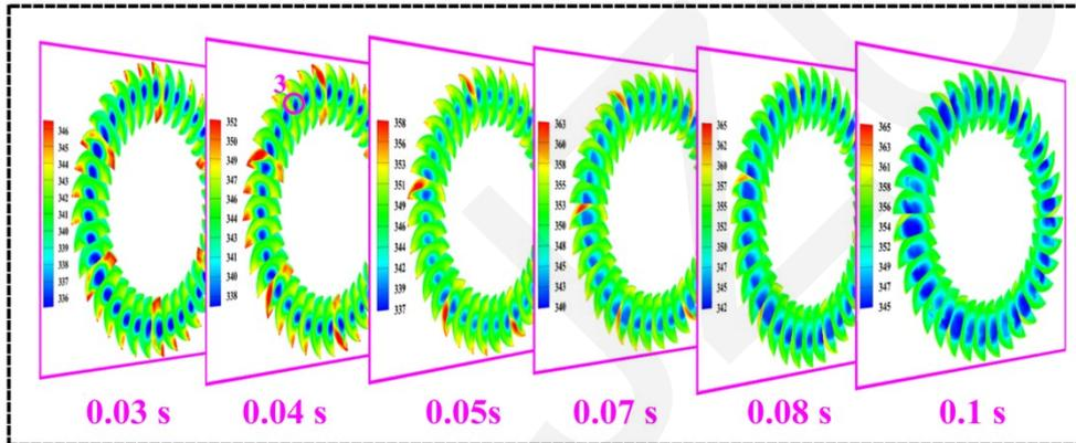
**Fig. 3** Temperature evolution cloud over time on the pressure blades.
