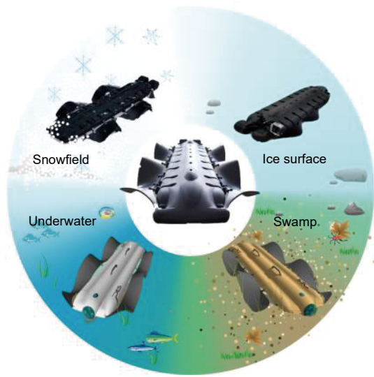
Fig. 4 Velox robot in different environments. The robot can not only march on the ground, underwater, and on sand, but also move on snow, asphalt roads, and ice (PES, 2017)
