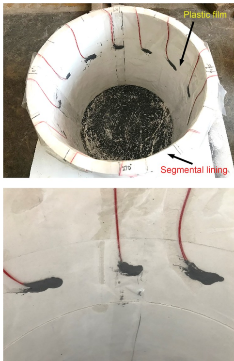
Fig. 7 Modelling of the lining–lining interface
