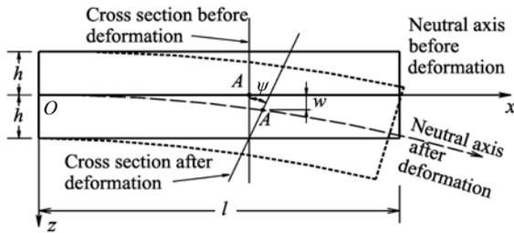
**Fig.1 Piezoelectric bimorph: coordinates and geometry**
