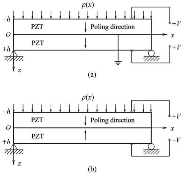
Fig.2 Piezoelectric bimorph settings: (a) parallel arrangement (Y-P); (b) series arrangement (X-P)
