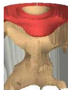
Fig.7 Solid-body contours of gas hold-up for gas-liquid mixing
