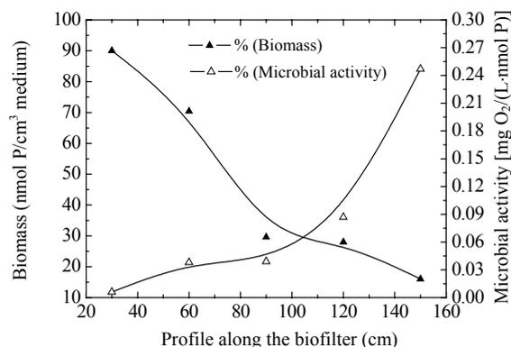
Fig.6 Biomass and microbial activity along the biofilter
