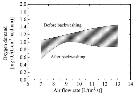
Fig.9 The average oxygen demand of biofilter before and after backwashing
