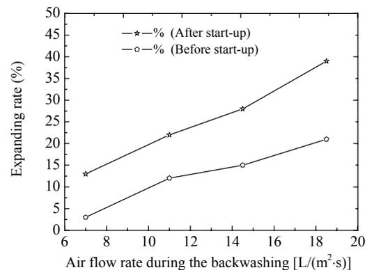
Fig.4 Change of expanding rate of filter with different air flow rate during backwashing
