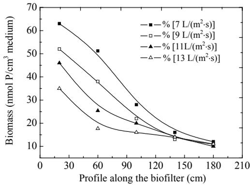
Fig.7 Change of biomass along the biofilter with different air velocity during backwashing
