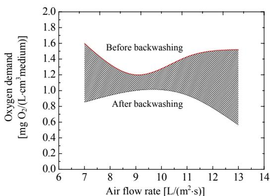
Fig.5 Oxygen demand before and after backwashing
