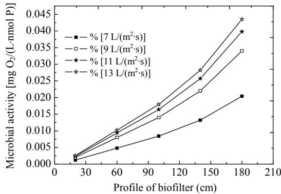
Fig.8 Change of microbial activity along the biofilter with different air velocity during backwashing
