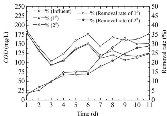
Fig.2 Effect of backwashing on the start-up of biofilter
