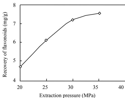
**Fig.3 Effect of the pressure on the yield of flavonoids**
