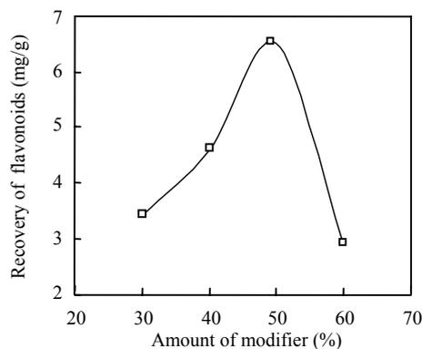
**Fig.1** Effect of amount of ethanol added on the yield of flavonoids
