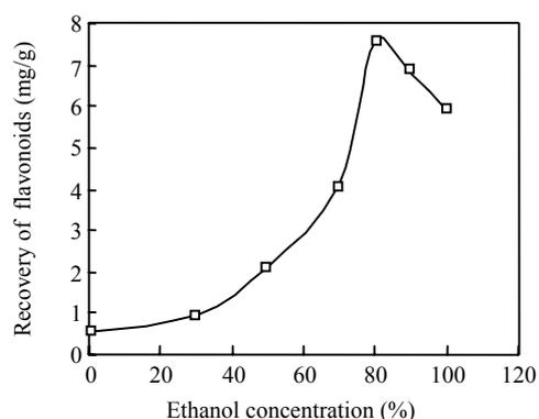
**Fig.2** Effect of ethanol concentration on flavonoids recovery
