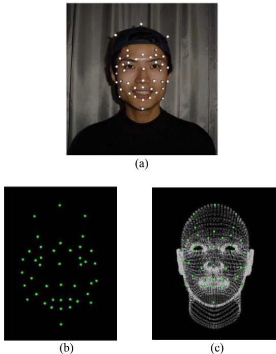
**Fig.1** Correspondences between markers and head model vertices are made manually or with the aid of some heuristic search. (a) Facial motion performer with 42 markers (Including 3 markers for global motion estimation); (b) Facial motion data captured by MoCap device; (c) Deformable head model (in vertex rendering context) with markers mapped onto it
