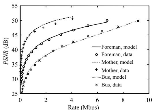
**Fig.2 Rate-PSNR performance of Foreman, Mother and Daughter, and Bus CIF sequences, all encoded using H.264/AVC at 30 frames/s, with GOP length of 15. The experimental data points are fitted with the model curve**
