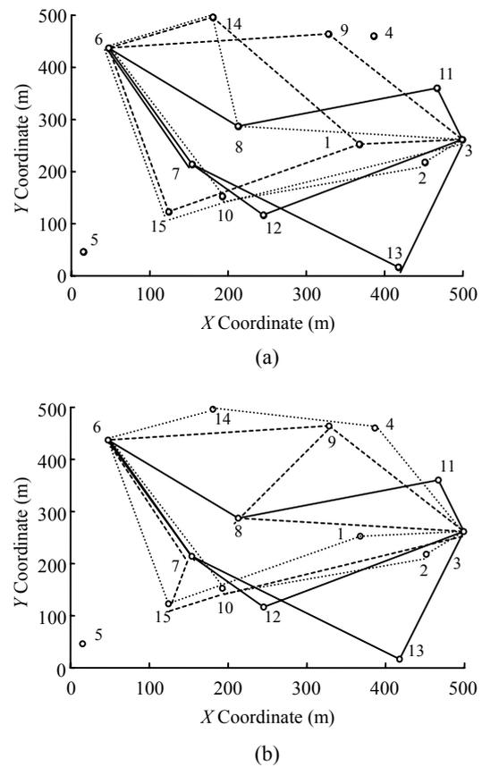
**Fig.5** (a) Initial and (b) final route selections of all three streams: Foreman in solid line, Mother and Daughter in dashed line and Bus in dotted line. Two routes for Mother and Daughter and three routes for Bus have changed over the iterations. For this instance, the  $\lambda$  in Eq.(8a) is chosen to be 0.1, and the rate increment is 100 kbps
