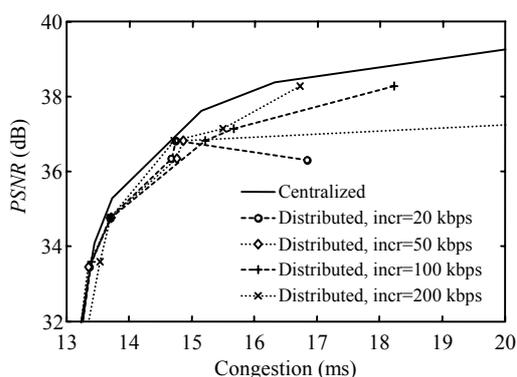
Fig.7 Trade-off between overall network congestion in terms of average link delay and average video quality of all three video streams in PSNR, using the proposed distributed joint routing and rate allocation algorithm. The performance of the centralized solution is also plotted in solid lines for reference
