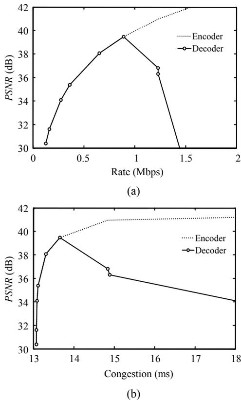
**Fig.4** Encoded and received video quality in PSNR versus (a) allocated rate and (b) network congestion in terms of average link delay, when streaming the Foreman sequence over the network using joint routing and rate allocation
