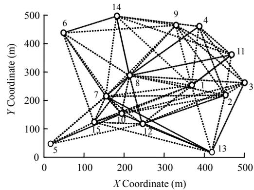
**Fig.1 Example network with 15 nodes randomly positioned in a 500 m-by-500 m square area. Dashed lines indicate the link between two neighboring nodes. All three video streams are sent from Node 3 to Node 6**
