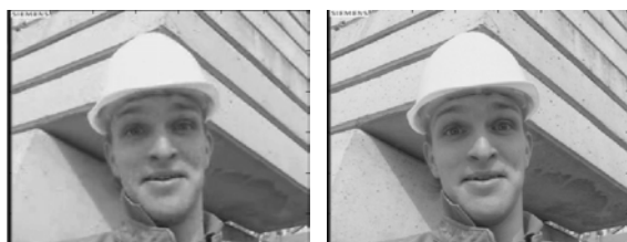
(a) Mode 1, 700 kbps, PER=0, PSNR=37.07 dB (b) Mode 5, 4235 kbps, PER=0.04, PSNR=44.85 dB
