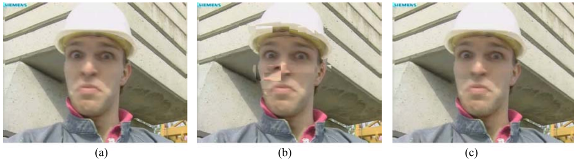
Fig.7 Decoded frames from the Foreman sequence at a symbol error probability of 10^{-4} . 100 kbps of FEC fails to correct the channel errors, reducing the picture quality. At the same bit rate, SLEP replaces the lost portions by their Wyner-Ziv decoded redundant counterparts and ensures acceptable picture quality. The 2 dB difference between the error-free picture and the picture decoded by SLEP is due to the quantization mismatch from Wyner-Ziv decoding. (a) Error-free: 41.10 dB; (b) FEC: 28.03 dB; (c) SLEP25: 39.12 dB
