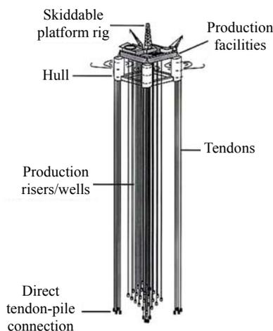
**Fig.1 Configuration and components of tension leg platform (Source: the Internet)**
