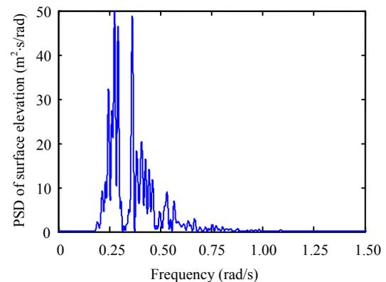
Fig.4 PSD of surface wave
