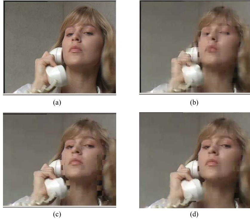
Fig.3 Miss CIF (frame P0). (a) Original image; (b) Restored by bilinear interpolation; (c) Restored by JM86; (d) Restored by Proposal 2
