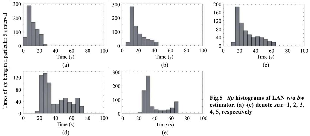
**Fig.5** *ttp* histograms of LAN w/o *bw* estimator. (a)–(e) denote *size*=1, 2, 3, 4, 5, respectively
