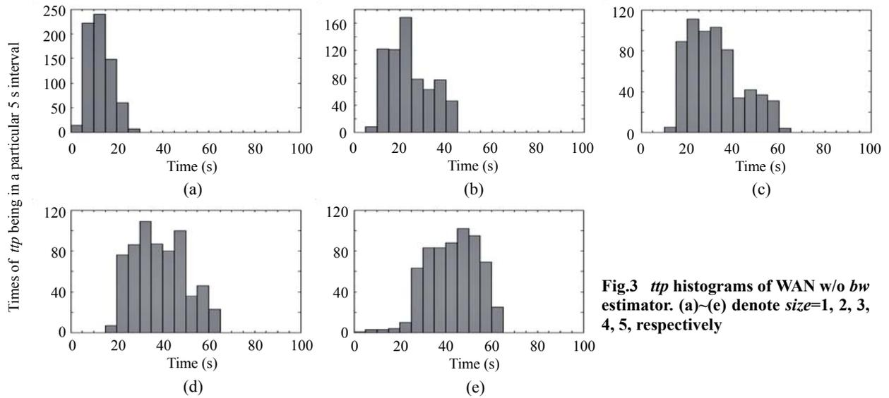
**Fig.3**  $ttp$  histograms of WAN w/o  $bw$  estimator. (a)~(e) denote  $size=1, 2, 3, 4, 5$ , respectively
