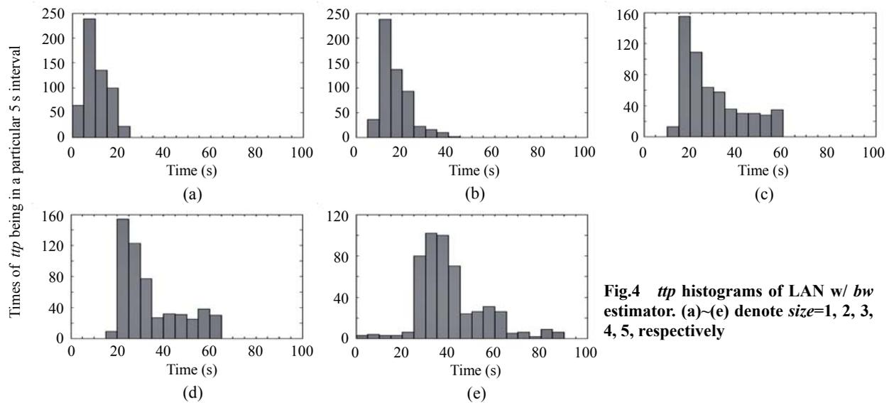
**Fig.4**  $ttp$  histograms of LAN w/  $bw$  estimator. (a)~(e) denote  $size=1, 2, 3, 4, 5$ , respectively
