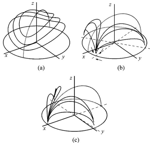
Fig.3 Fiber orientation orbits in shear and extension combined flow. (a)  $k=-0.5, j=-0.5$ ; (b)  $k=0.5, j=0.5$ ; (c)  $j=10$ . The dash lines in (b) and (c) denote the approximation directions. Orbits in (c) is the approximation of almost-extension flow case
