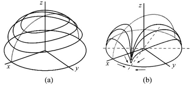
Fig.2 Fiber orientation orbits in double shear flow
