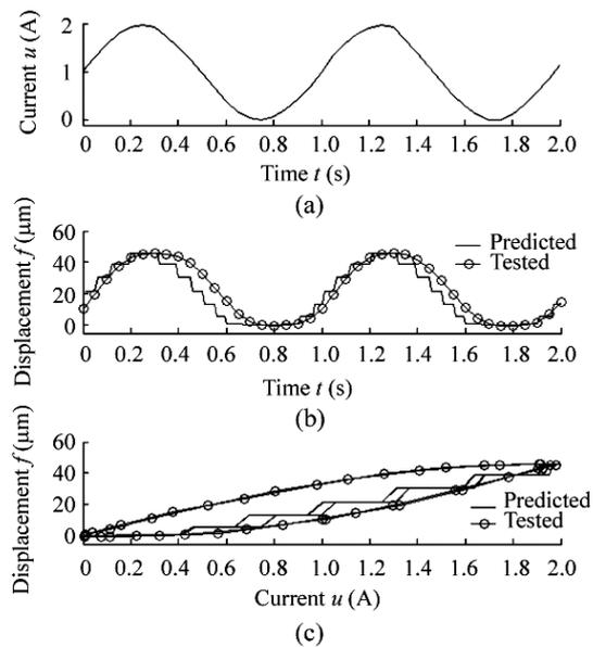
Fig.8 Predicted and tested results by DFM. (a) Driven current waveform to the GMA; (b) Predicted and tested displacement waveform by DFM; (c) Predicted and tested hysteresis loop by DFM
