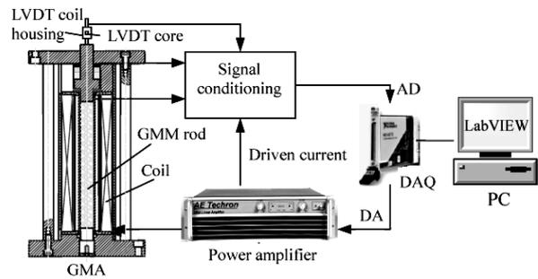
Fig.4 Schematic drawing of the experimental system
