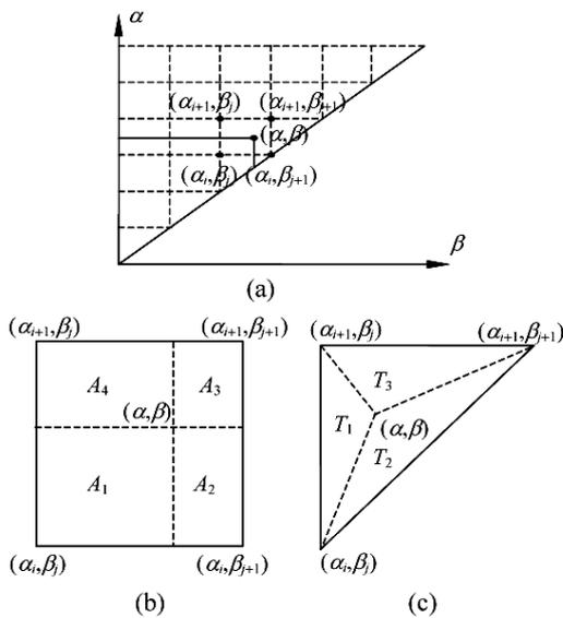
**Fig.10** Illustration of 2D interpolation. (a) The big triangle region in Preisach plane; (b) The point drop in the rectangle region; (c) The point drop in the triangle region
