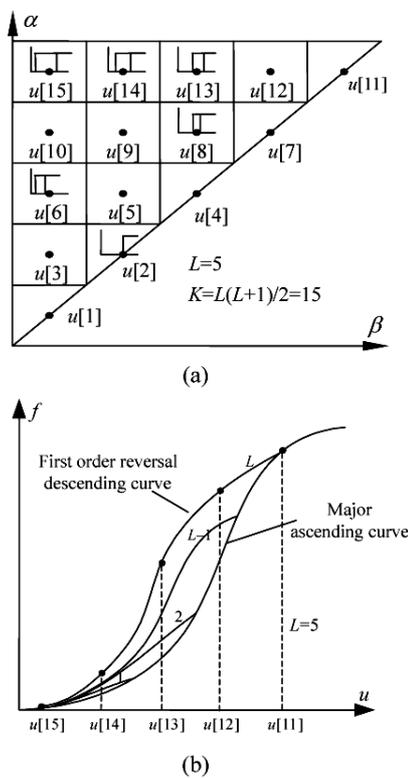
**Fig.1 Discretization of Preisach plane. (a) Preisach plane; (b) The discretization points on the reversal descending curve**
