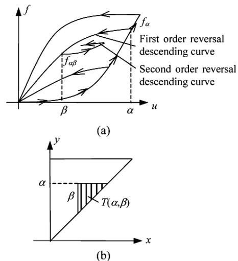
**Fig.2 Geometrical interpretation of  $F$  function. (a) First and second order reversal descending curve; (b) The formation of triangle region in Preisach plane**
