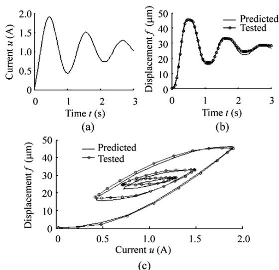
**Fig.12 Predicted and tested result of high order curves. (a) Variation of the driven current's amplitude; (b) Predicted and tested displacement waveform; (c) Predicted and tested high order hysteresis loop**
