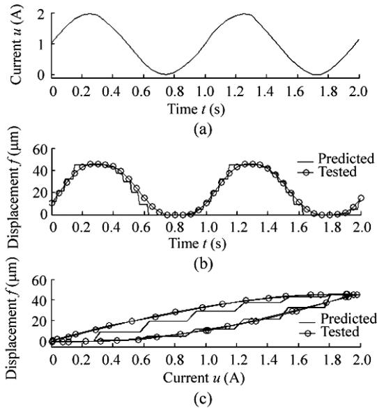
**Fig.9** Predicted and tested results by FFM. (a) Driven current waveform to the GMA; (b) Predicted and tested displacement waveform by FFM; (c) Predicted and tested hysteresis loop by FFM
