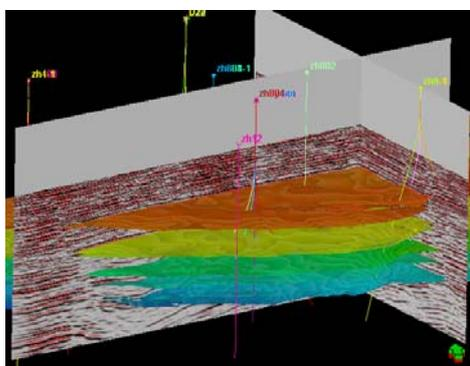
Fig.2 The correlation chart of time fault structure model and seismic cross section
