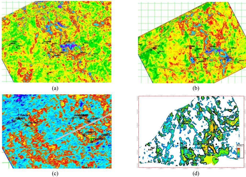
Fig.5 The correlation of geological model sand body NmIII2 isopach and seismic property parameter (NmIII2 is horizon name). (a) The mean-square-root amplitude; (b) Average shale content by seismic inversion; (c) Seismic pre-stack average Poisson ratio; (d) Geological model isopach chart of sand body
