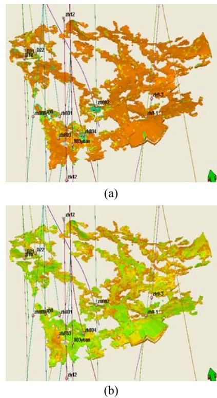
Fig.7 3D display of NmIII2 porosity model (a) and permeability model (b)
