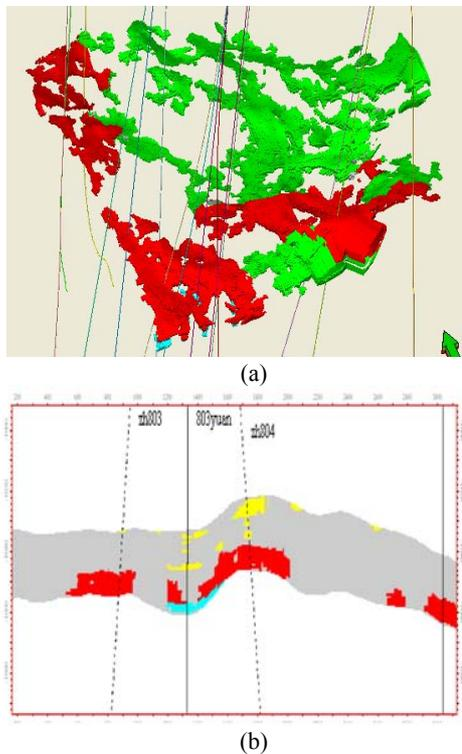
Fig.6 NmIII2 small oil layer interpretation fruit chart. (a) 3D display of oil layer distribution; (b) Oil layer distribution across well cross section
