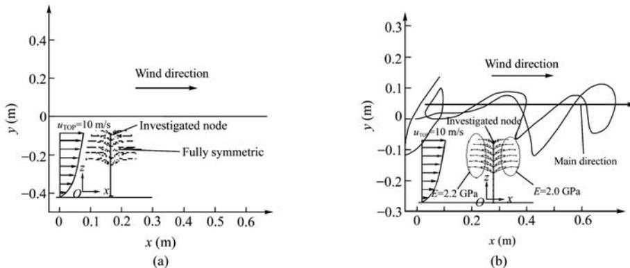
Fig.8 Sample of motion for the investigated node of the FE tree model-II. (a) With fully symmetric condition; (b) With asymmetric branch elasticity
