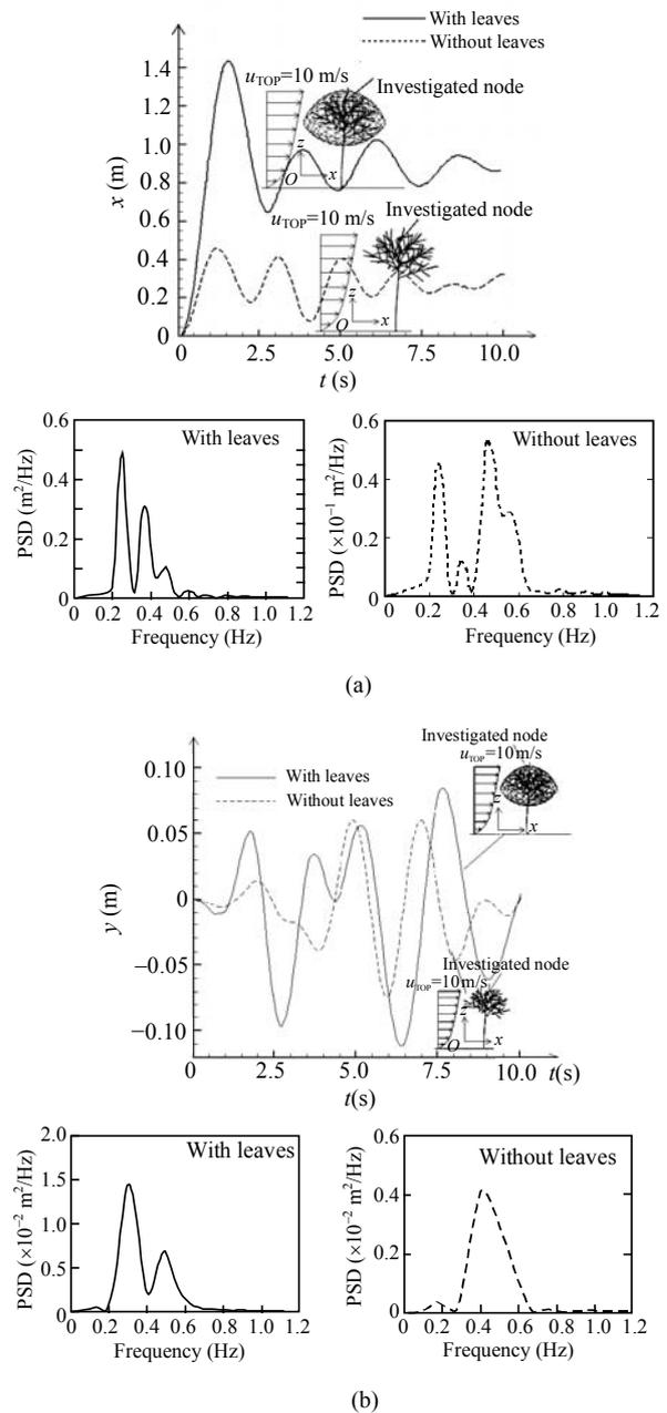
**Fig.10 Comparison of  $x$  displacement (a) and  $y$  displacement (b) With and without leaves (model-I)**
