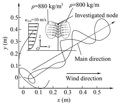
**Fig.9 Sample of motion for asymmetric branch density (model-II)**
