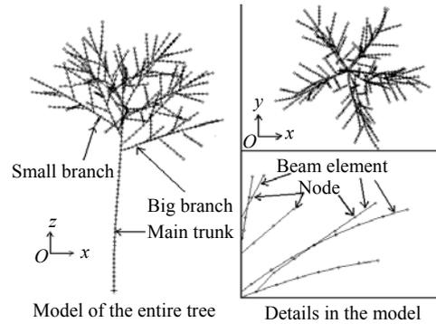
Fig.1 FE tree model-I (asymmetric model)
