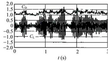
Fig.3 Drag ( $C_D$ ) coefficient and lift coefficient ( $C_L$ ) at Reynolds number  $6.1 \times 10^4$  (Nishimura and Taniike, 2001)
