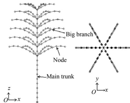
Fig.2 FE tree model-II (symmetric model)
