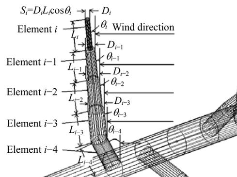
Fig.4 Wind force calculation
