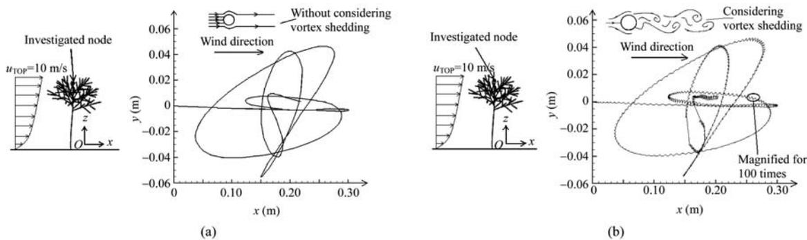
Fig.7 Sample of motion for the investigated node of the FE tree model-I. (a) Without vortex shedding; (b) With vortex shedding
