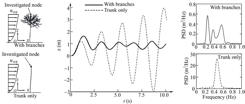
Fig.11 Tree with branches and trunk only in fluctuating wind (model-I)
