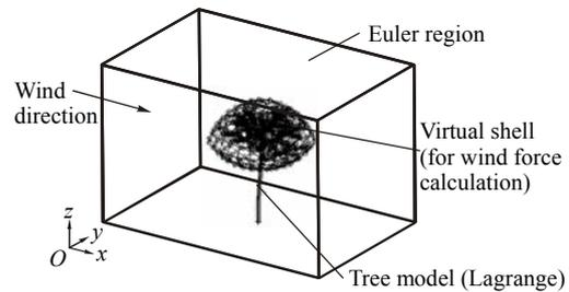
Fig.6 FSI analysis of the FE tree model-I with leaves
