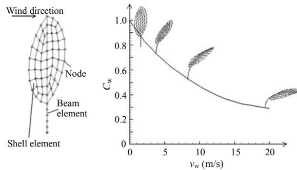
Fig.5 FE simulation result of a leaf in wind field
