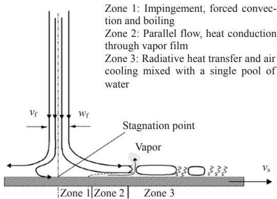
Fig.2 Heat transfer in water cooling area
