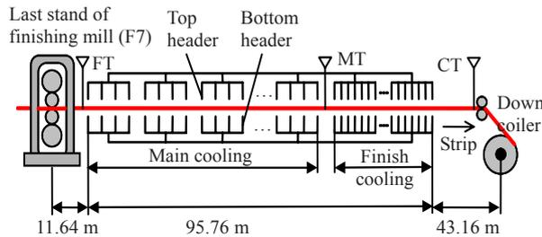
Fig.1 Schematic diagram of the ROT
