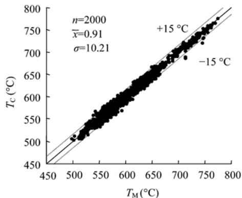
**Fig.8 Comparison between measured coiling temperature and calculated coiling temperature**
