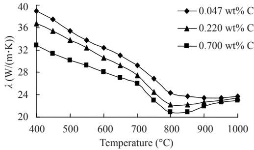
Fig.4 Steel conductivity as function of temperature
