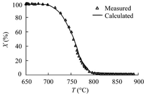
**Fig.7 Comparison between measured and calculated volume fraction of ferrite during cooling**
