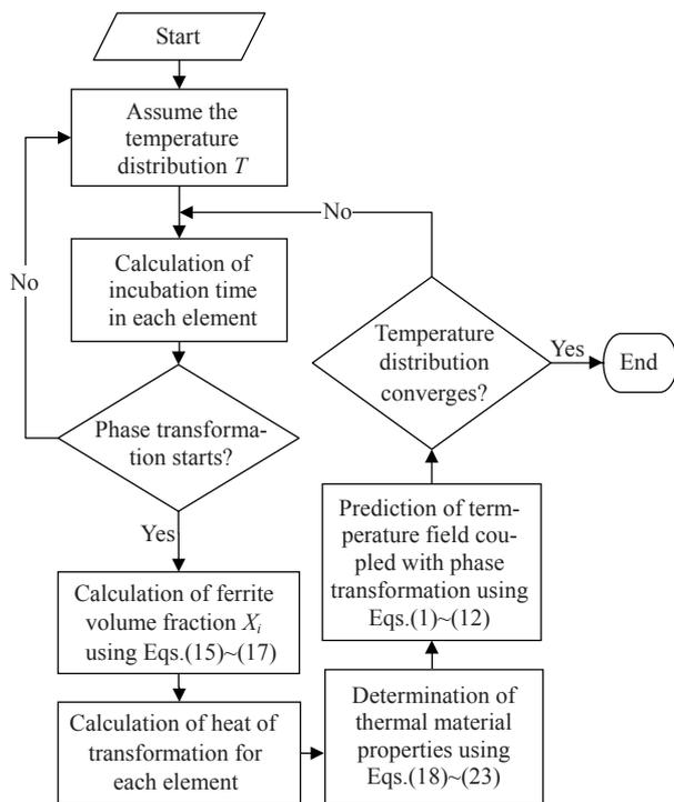
Fig.3 Iterative procedure for solving heat transfer and phase transformation
