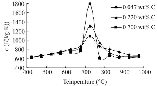
Fig.5 Steel specific heat as function of temperature
