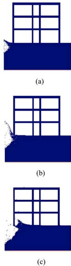
Fig.9 Simulations of subsurface blast processes. (a) t=3.8 ms; (b) t=15.0 ms; (c) t=82.6 ms
