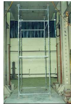
Fig.5 Installation of a 2-story system scaffold without diagonal braces before loading
