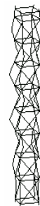
Fig.17 Deformation shape of an 8-story system scaffold (Case B in Fig.15) after loading (BC: hinge; joint stiffness: 785 kN·cm/rad)
