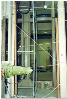
Fig.7 Deformation shape of a 2-story system scaffold without diagonal braces
