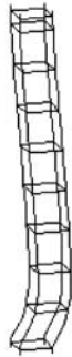
Fig.14 Deformation shape of an 8-story system scaffold after loading (BC: hinge; joint stiffness: 785 kN·cm/rad; joint position: Case A in Table 1)
