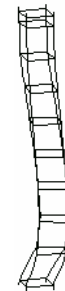
Fig.20 Deformation shape of an 8-story system scaffold (Case B 2 in Fig.18) after loading (BC: hinge; joint stiffness: 785 kN·cm/rad)
