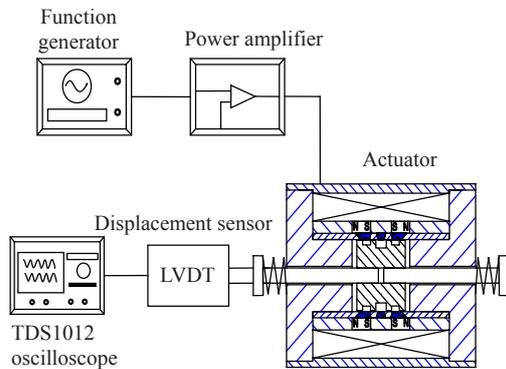
Fig.4 Schematic of the experimental system
