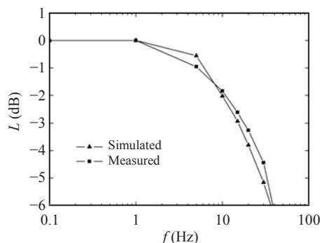
Fig.6 Comparison between the simulated and experimental frequency response characteristics
