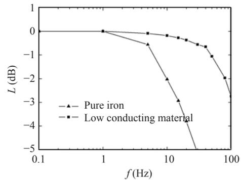
Fig.3 Simulated frequency response of the actuator adopting two different magnetic materials
