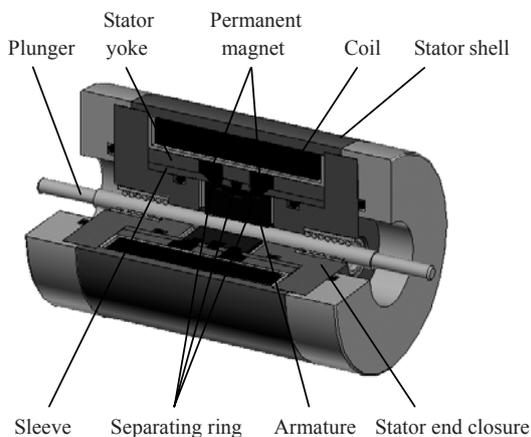
Fig.1 Structure of the actuator
