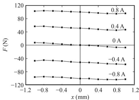
Fig.2 Static force-versus-displacement characteristics
