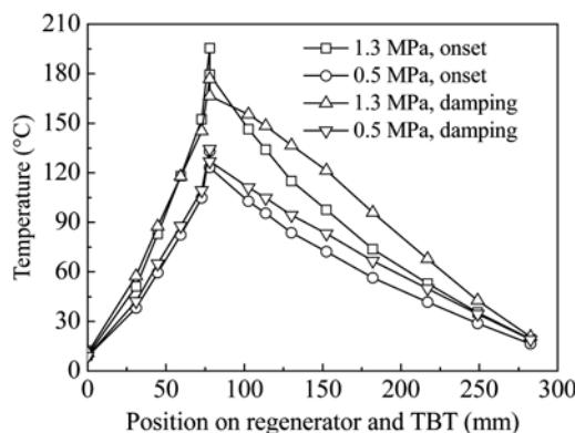
**Fig.8 Temperature distribution along regenerator and TBT for onset and damping process at relatively low heat input (50 W at 0.5 MPa, 100 W at 1.3 MPa)**
