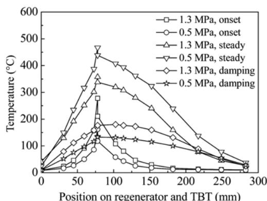
**Fig.9 Temperature distribution along regenerator and TBT during onset, steady state and damping at relatively high heat input (500 W at 0.5 MPa, 800 W at 1.3 MPa)**
