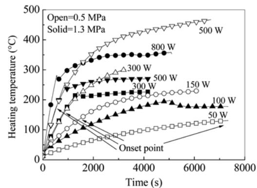
**Fig.7** Heating-up process at different heat inputs
