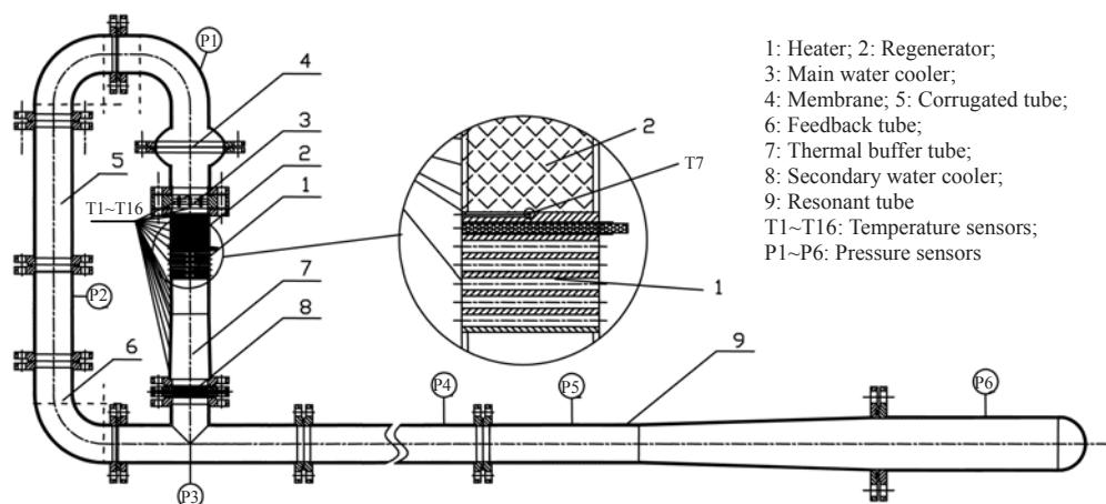
Fig.1 Schematic of traveling-wave thermoacoustic prime mover
