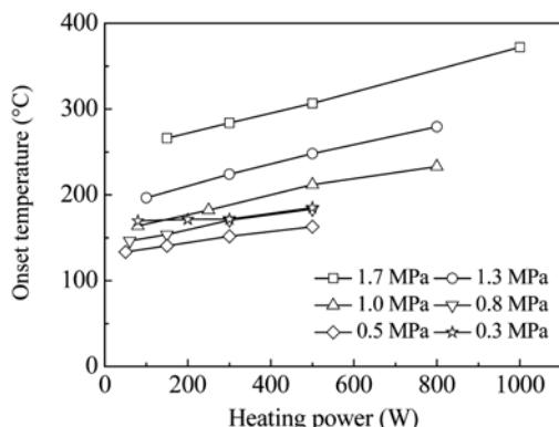
**Fig.4** Onset temperature vs heating power at different filling pressures
