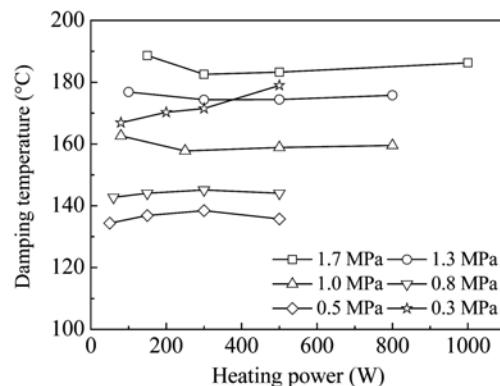
**Fig.5** Damping temperature vs heating power at different filling pressures
