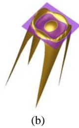
Fig.1 Region segmentation of a B-spline surface (a) A biquartic B-spline surface with peak (red), pit (green), and saddle (yellow); (b) The scalar field surface of \Psi with its zero set
