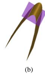
Fig.2 Region segmentation of developable surface (a) A developable surface with ridge (pink) and valley (blue); (b) The scalar field surface \Phi with its zero set
